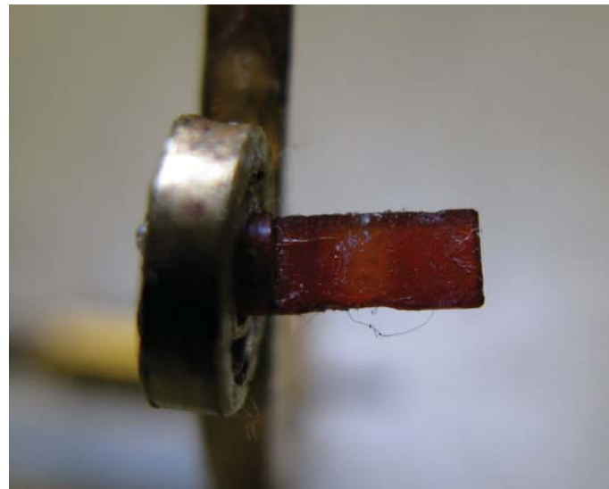
3. Definitely not a sliding fit in the hole!
