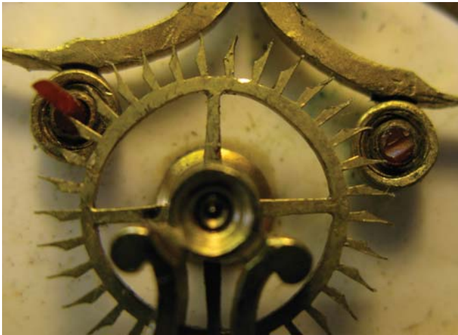
1. An example of the very rare 'Tocorb' escapement..
