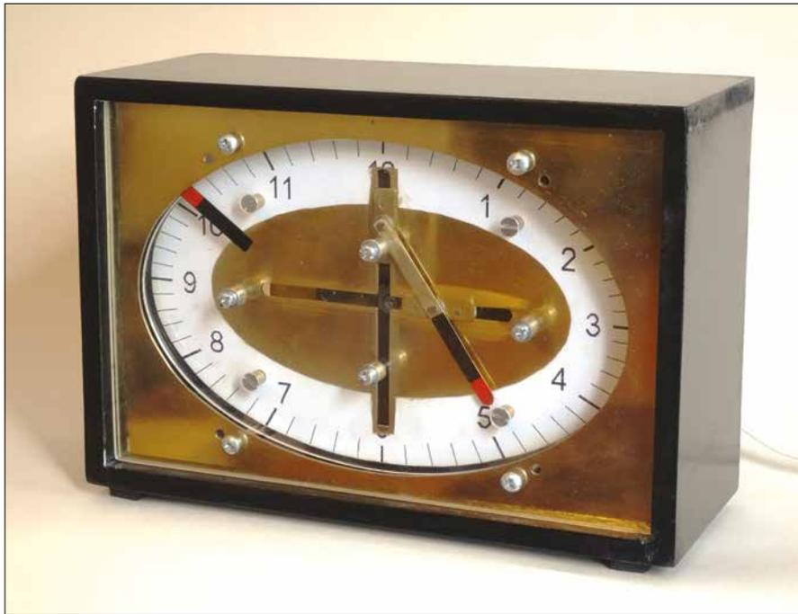
Figure 2. The elliptical clock indicating 4:51.
