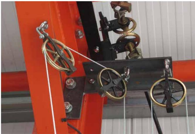
Figure 5. Bevel gears taking drive to the drum, together with the weight cord and pulleys.
