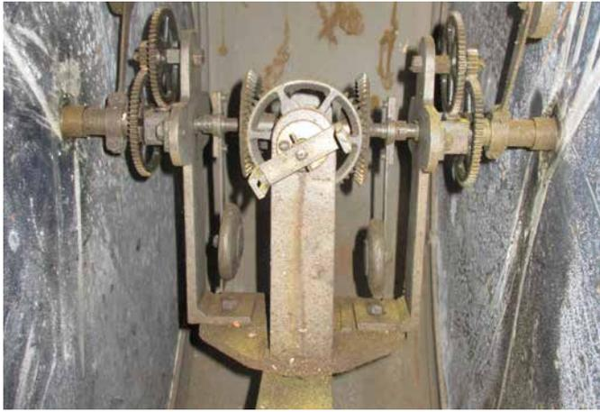
Figure 3. Dial-works of drum.
