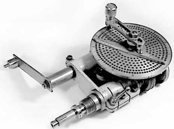
Figure 3. The parts fitted to the Myford dividing head.
