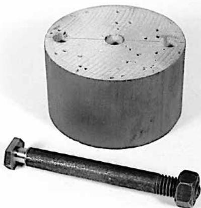
Figure 8. The packing piece to raise the vertical slide.
