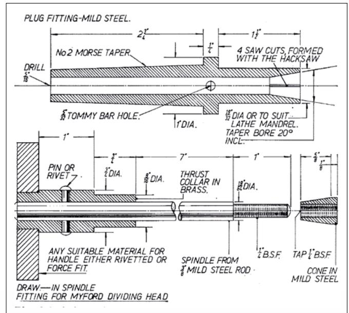
Figure 1. Drawings of parts required to fit Myford dividing head to Myford headstock.
