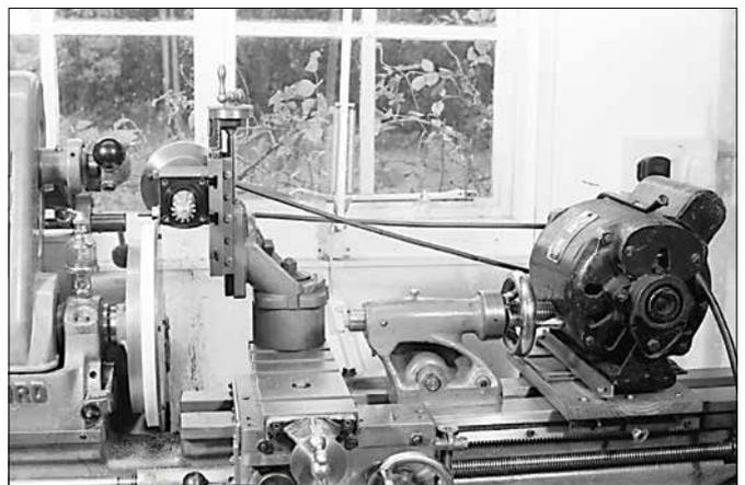
Figure 9. Method of driving the milling spindle.
