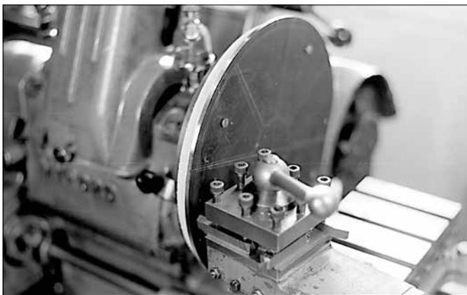
Figure 6. Turning the brass blank (CZ120) to size.
