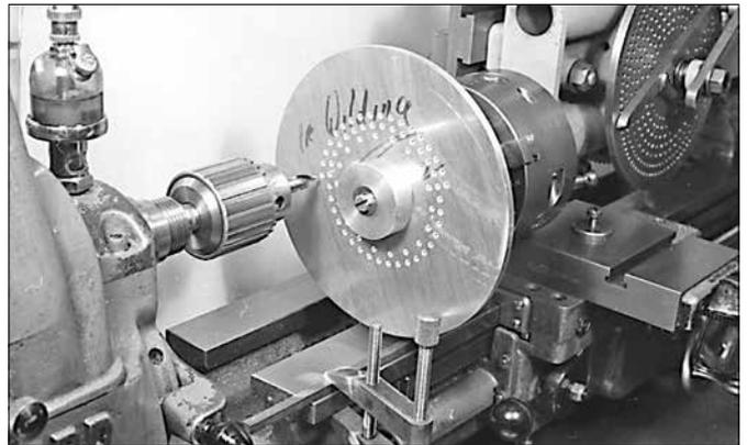
Figure 5. Drilling holes in a special plate using the dividing head.
