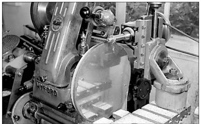
Figure 7. Cutting the 290 teeth.
