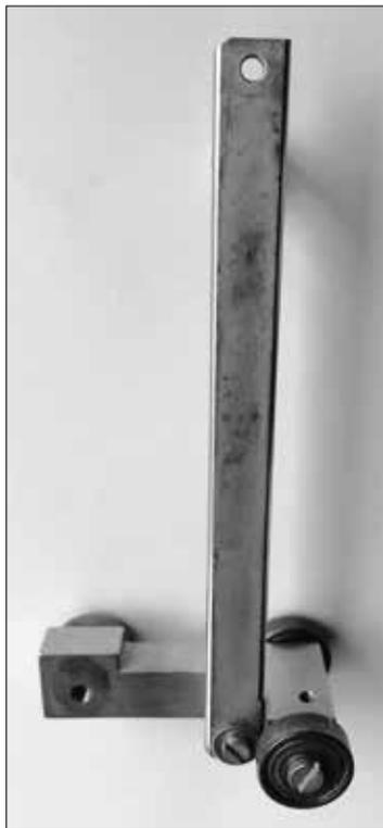
Figure 3. Details of the main carriage, with its three 22mm sealed, steel ball races that serve as wheels, and the vertically mounted precision, steel slider bar; the hole at the upper end is for item k in Figure 2.
