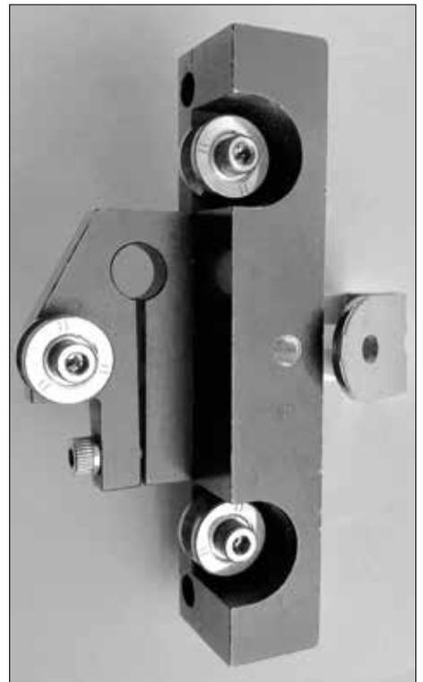
Figure 4. The sliding carriage to which the screw holder is attached. Note the screw (g in Figure 2) for adjusting the rolling tension of the ball races.
