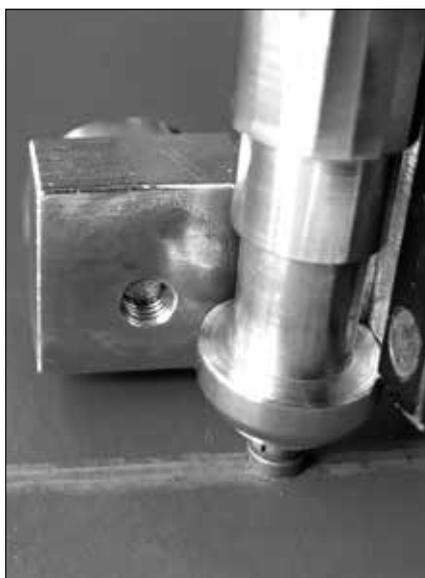
Figure 5. Close up of a screw head being drawn across 1200-grit Emery paper that rests on a glass platen. Note the streak of iron filings on the paper.
