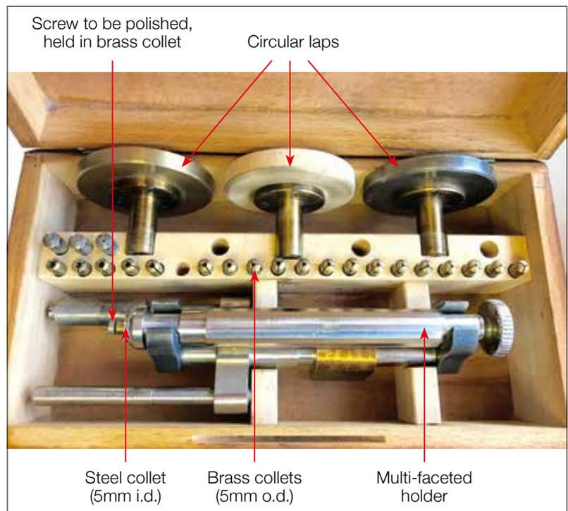
Figure 1. Lorch-Schmidt screw head polishing tool.
