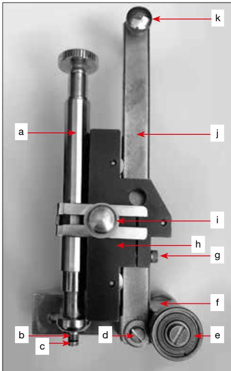
Figure 2. The new type of screw head polisher
