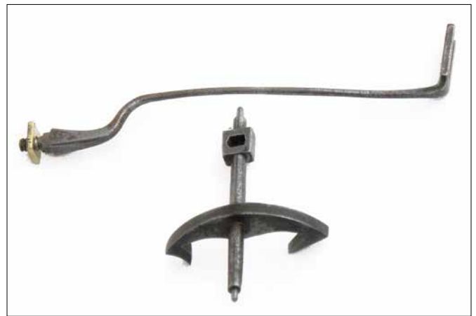
Figure 7. The anchor escapement and removable crutch.
