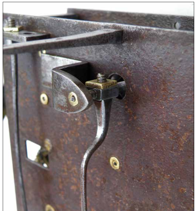
Figure 8. The backcock and support for a thread pendulum suspension.
