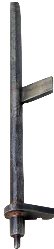
Figure 11. Detail of the hammer flag and the combined arm for the spring and stop.
