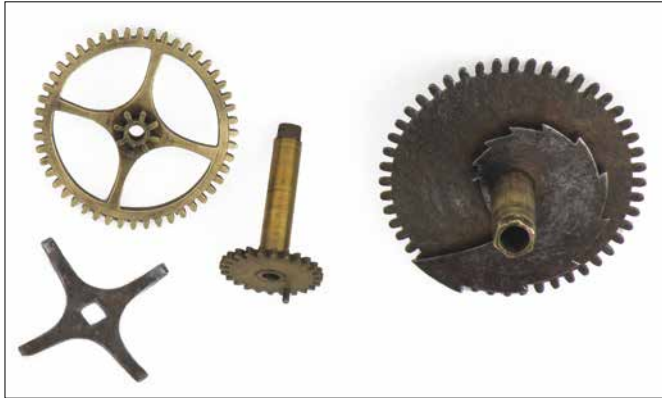
Figure 3. The motion-work with an iron hour wheel and iron snail.
