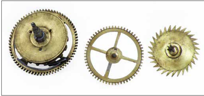
Figure 2. The three wheels of the going train.
