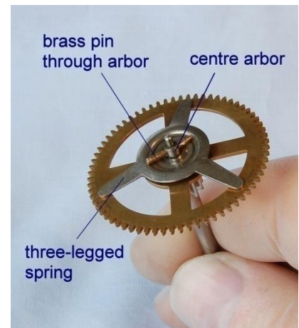
Figure 90 – the components of the friction drive
