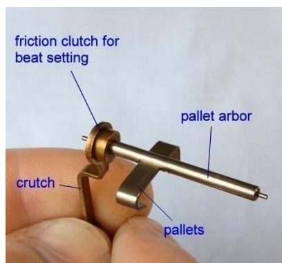
Figure 69 – pallet assembly
