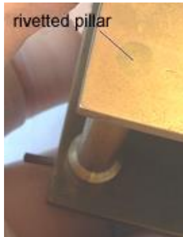
Figure 99 – pillar rivetted to back plate
