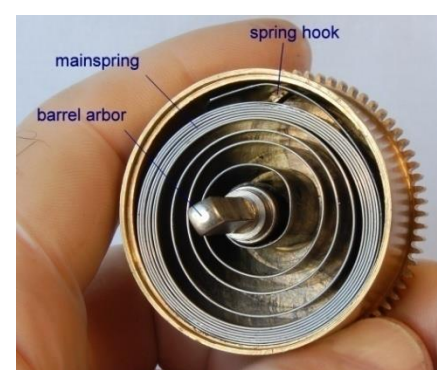
Figure 84 – barrel with end cap removed
