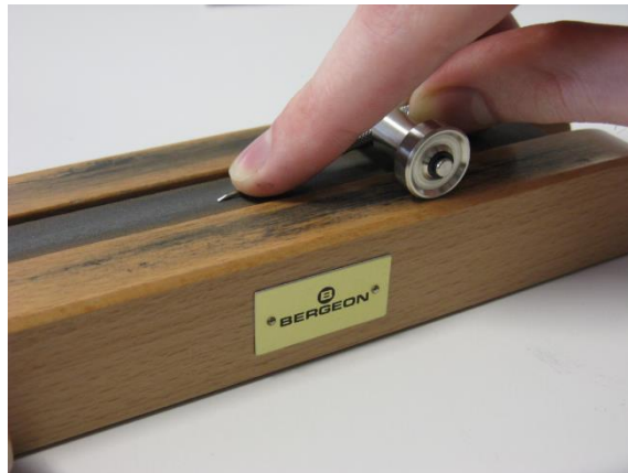
Figure 109 – using a screwdriver sharpening device
