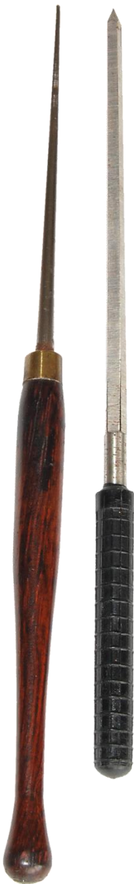
Figure 131 – smoothing broach (left), and cutting broach
