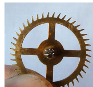
Figure 88 – tooth form of escape wheel
