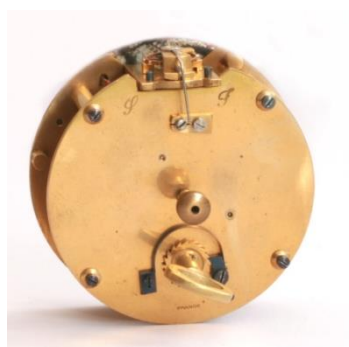
Figure 20 – drum movement showing platform escapement
