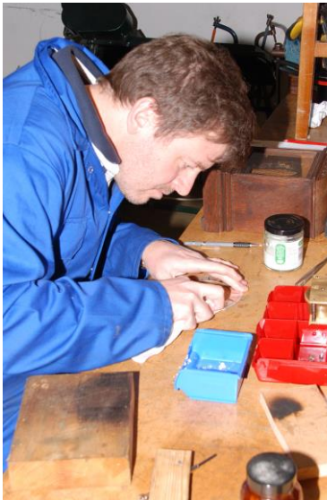
Figure 10 – silvering a chapter ring in the BHI clock workshop
