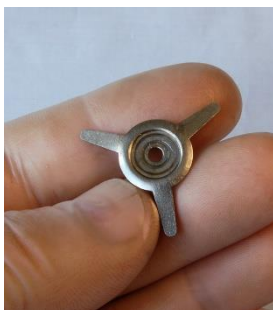
Figure 91 – three-legged friction spring
