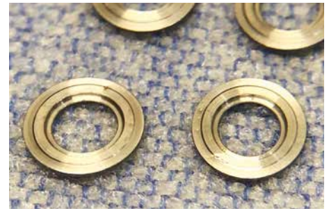
Figures 3A and B. In the 'Gearing' department, these steel blanks will become ratchet wheels. Due to the boss on their underside, these cannot be stacked and must be hobbled one at a time. The wishbone delivers jets of cutting fluid, whilst a pointed cutter in the foreground slices burrs off the work.
