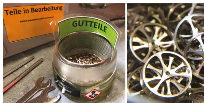
Figures 2A and B. Cupro-nickel balances, fresh off the sliding-head lathe.
