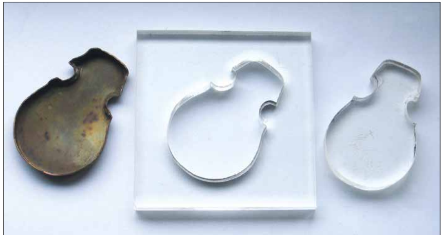
Figure 3. Perspex profile and trial pressing in gilding metal
