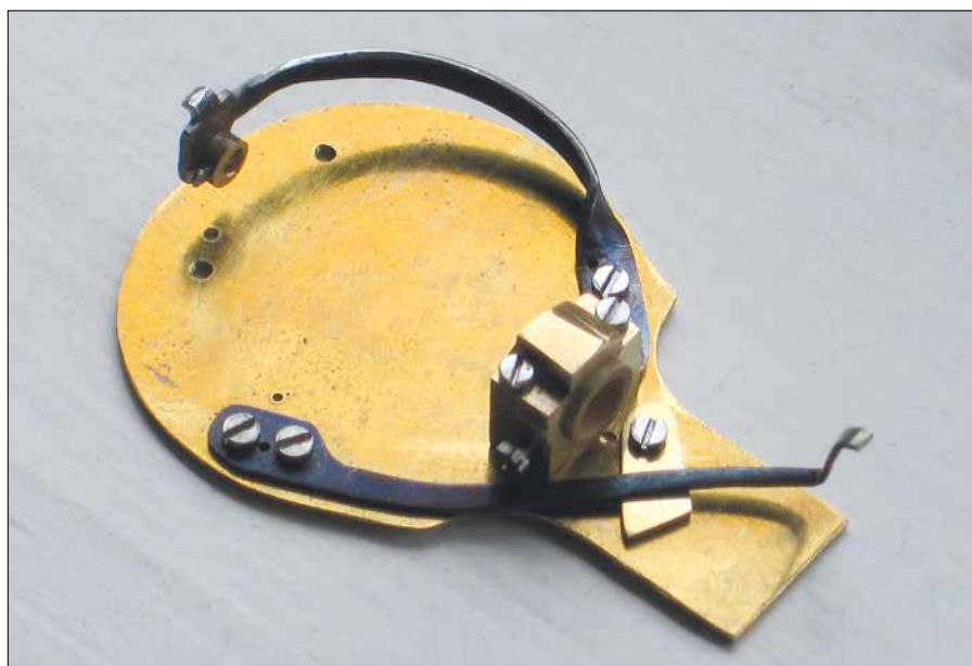
Figure 12. Main base plate with lock and fly springs screwed in position.
