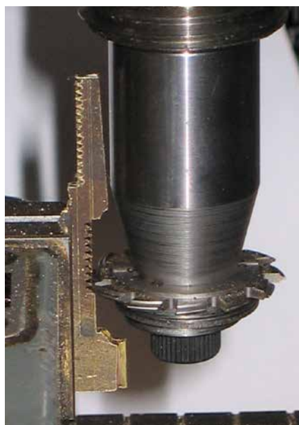
Figure 11. Milling teeth on second side of the rack.
