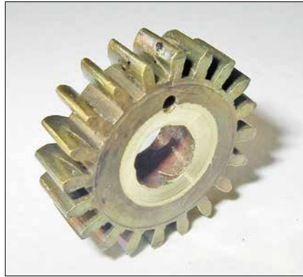
Figure 4. The original 20-leaf pinion with filed teeth and pockets of wear.
