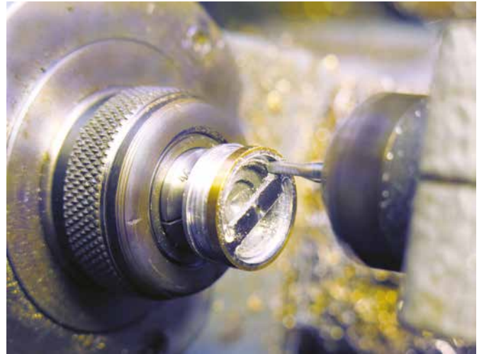
Figure 5. Milling the balance arm.
