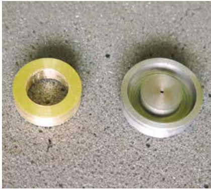
Figure 3. In making a new balance, a slot was turned in the steel disk, to be filled with a melted brass ring.
