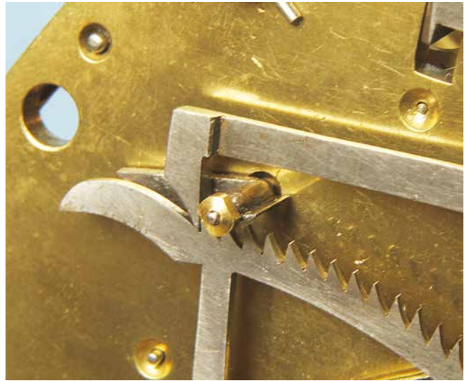
Figure 8B. A close up of the new retaining nut on the hour gathering pallet.
