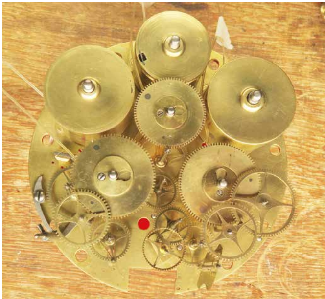
Figure 9. The movement part-assembled.
