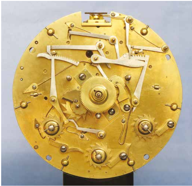
Figure 8A. The under-dial work. Several springs had to be made.
