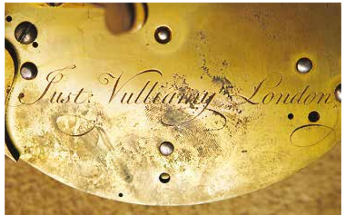
Figure 14. The back plate as received, including heavy fingerprint staining.
