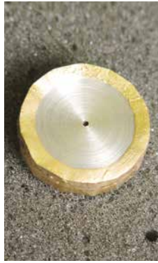
Figure 4. The balance after hammering the brass.
