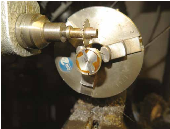
Figure 6. Slitting the balance rim.
