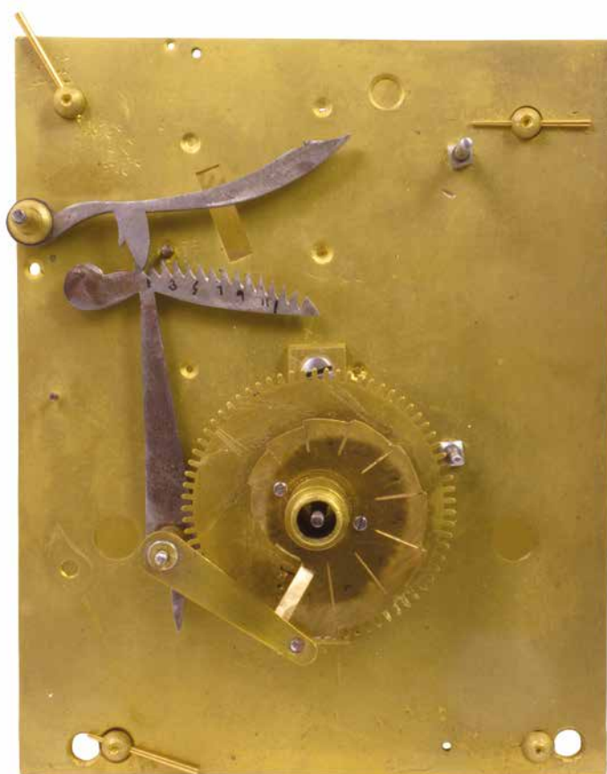
Figure 13. The finished snail and rack tail in place prior to cleaning up.
