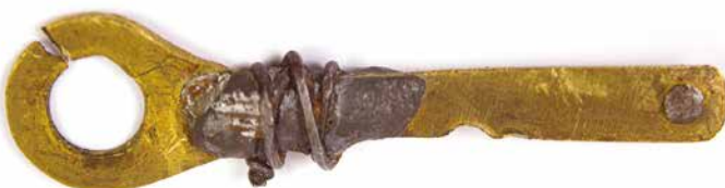
Figure 9. The old repaired rack tail.
