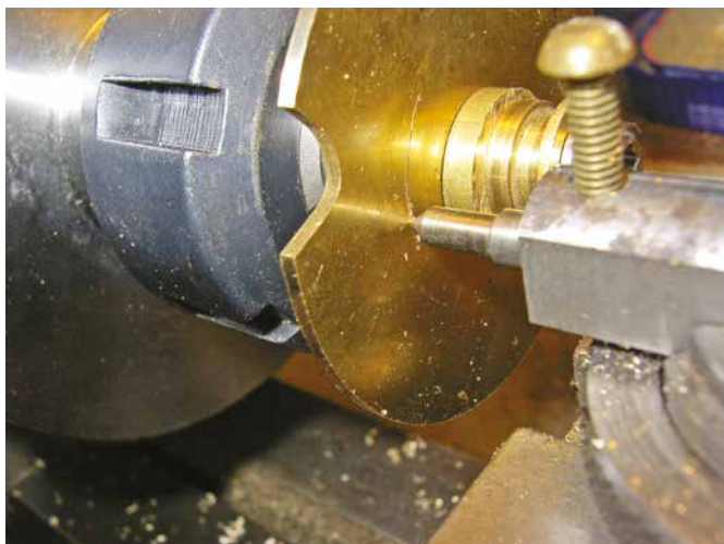
Figure 3. A circular mark for the 12 o'clock step position was made with the tool-post scribe.
