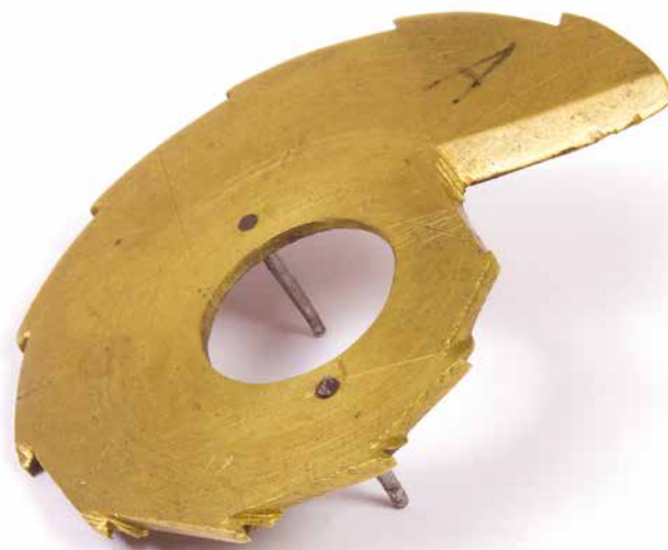
Figure 10. The six to 12 o'clock steps on the old snail had been cut down.
