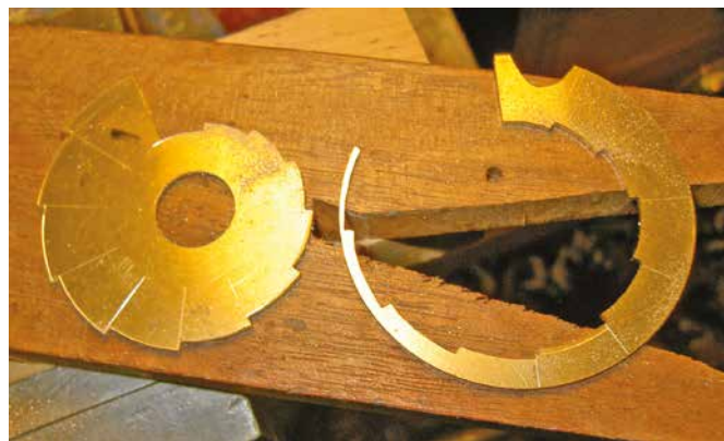
Figure 6. The snail profile was cut out using a piercing saw.
