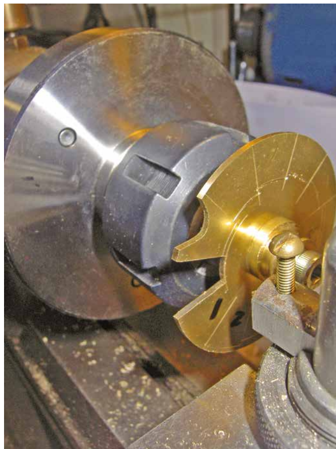
Figure 5. The tool-post scribe was used to mark each of the steps on the snail.
