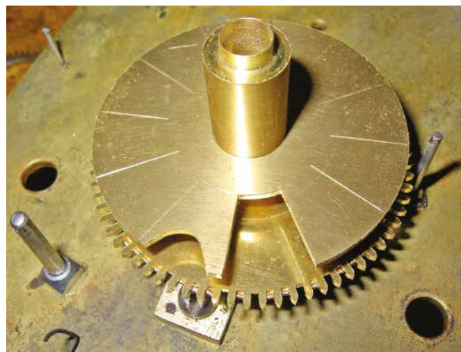
Figure 2. The snail disc was divided into 12 sectors. The last step on the snail was removed using a piercing saw. (The semi-circular cut-out is a leftover from another project).
