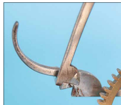
Figure 19. Strike locking block on release lever.
