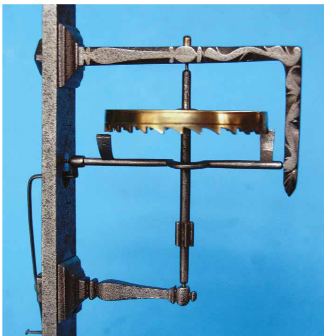
Figure 4. Comtoise escapement between potences.
