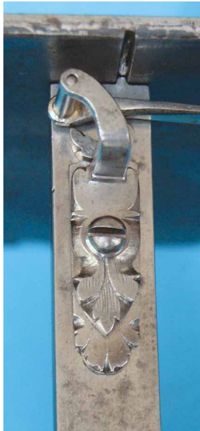
Figure 11. Clock frame post secured by a tenon in a groove. Also illustrates a decorated cock.
