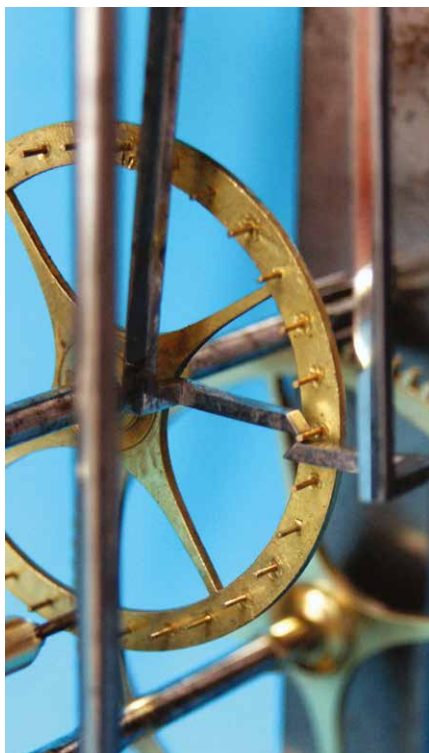
Figure 7. Comtoise pin wheel escapement.
