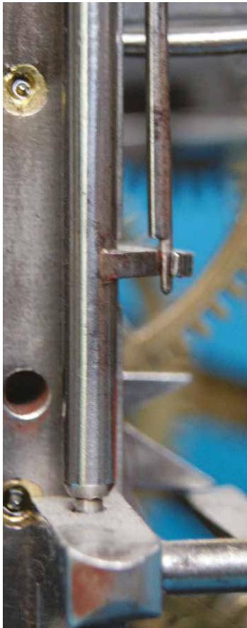
Figure 10. Notches on springs to hold hammer arbors in place.
