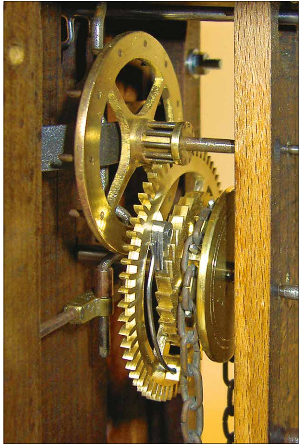
Figure 3. The new alarm great wheel, ratchet wheel, click, click spring and sprocket.
