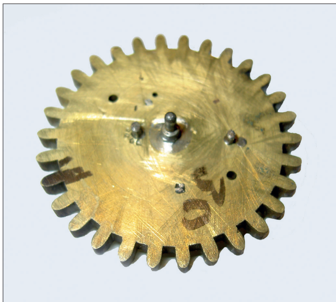
Figure 12. The canon wheel had multiple holes for let-off pins.
