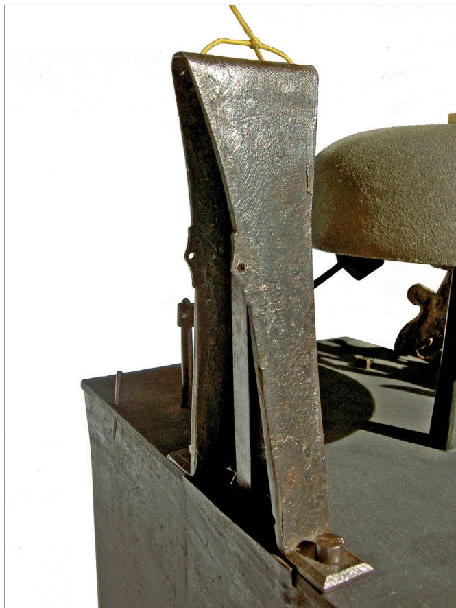
Figure 4. The tall suspension post for the rear pendulum. The rear cover, removed in this photo, is held in place with one long pin through the two holes.
