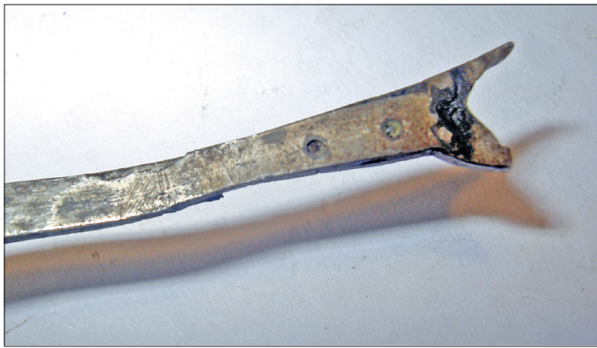
Figure 11. The detent with the added doe's foot.
