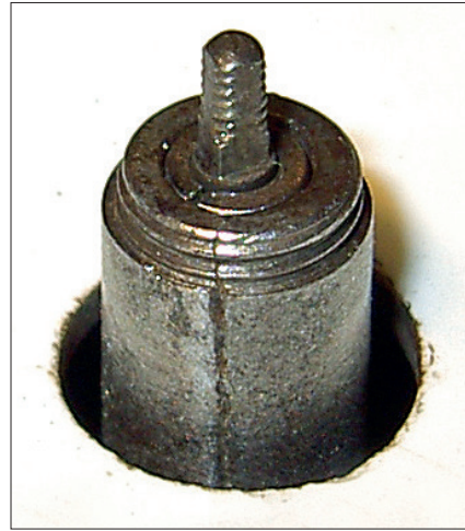
Figure 16. The thread on the nose of the steel hour pipe.
