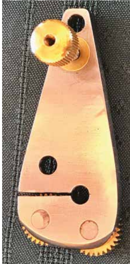
Figure 9. Distal side of the tumbler platform, showing the 4 mm knurled nut on its stud, used for locking the platform, and hence the tumbler wheels, into selected positions (forward, neutral and reverse motion of the slide rest relative to the lathe spindle).
