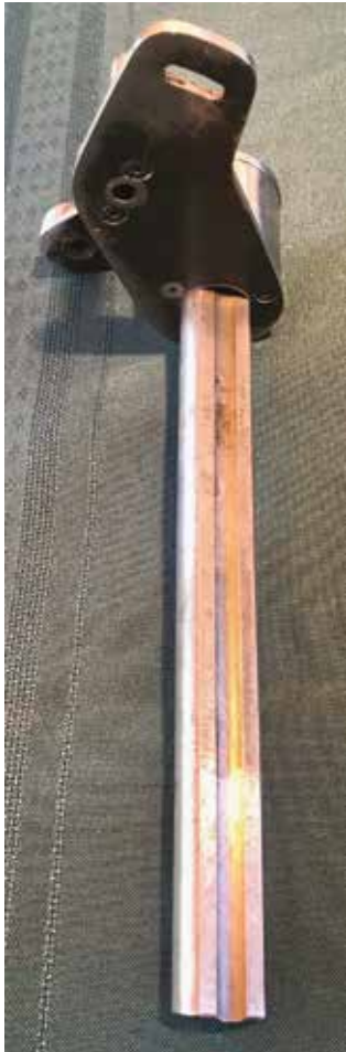
Figure 5. Back of the lathe's D-bed and the screw cutting attachment's proximal plate and main boss.
