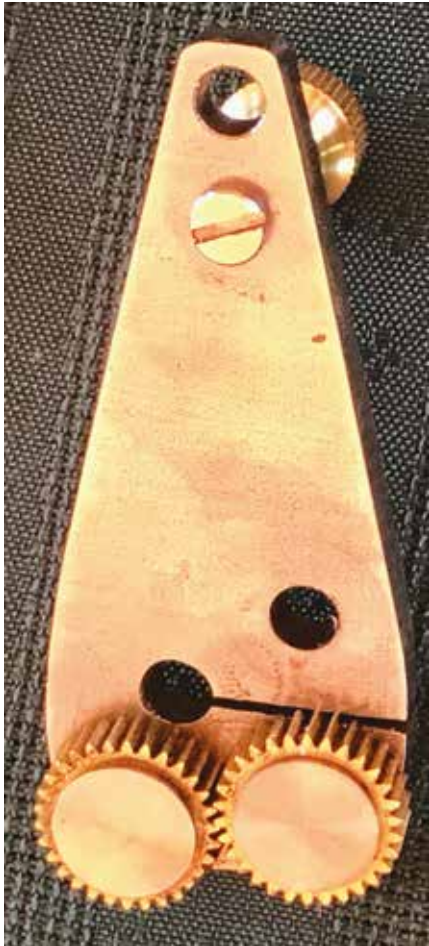
Figure 8. Tumbler wheels on their platform. Note the slit-and-hole used for fine adjustment of the depthing of the right-hand tumbler wheel with the 36-tooth wheel on the drive shaft.
