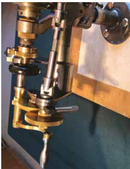
Figure 11. Side view, showing the universal joints on the feed screw shaft.
