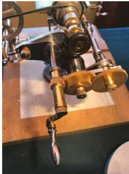
Figure 12. End view showing the crank and wheel train in detail. Here it is set up with a 25-tooth wheel driving a 95-tooth wheel that is linked on the banjo to a 60-tooth wheel that in turn drives a 90-tooth wheel. This gives a pitch ratio of 0.175.
