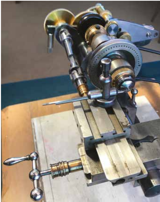
Figure 14. The cross slide with tool post and tungsten carbide graver sharpened to give the required thread profile on the cut screw.
