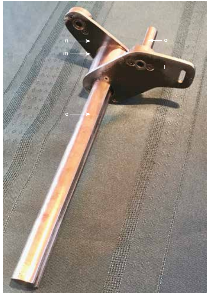
Figure 4. 20mm D-bed c with the main boss m and its two attached mounting plates; the proximal one l supports the drive shaft bearing o , while the distal one n supports the banjo and the feed screw shaft.
