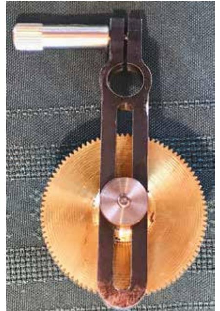
Figure 10. Banjo that supports the intermediate wheels. It fits, via the 11 mm hole, on to the feed screw bearing (shoulder) and is clamped into position by the long knurled nut. The banjo was cut from 5.75 mm blue steel with a CNC mill using a 3 mm tungsten carbide end-mill.
