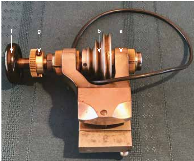
Figure 3. Wolf Jahn headstock a with its drive pulleys b located between the plain cone bearings; and the g drive wheel (0.5 module, 48 teeth involute profile) attached to the boss with three blued screws that clamp onto the spindle; and f the Bakelite drawbar knob.
