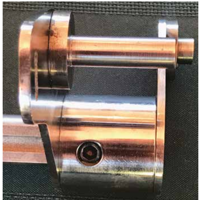
Figure 7. The silver steel main boss of 38 mm diameter, which is clamped on the D-bed via a single 9 mm socket-head cap screw tightened on to the rear groove. The boss has a central blind bored hole of 20 mm that extends to within ~5 mm of the end of its 35 mm length.
