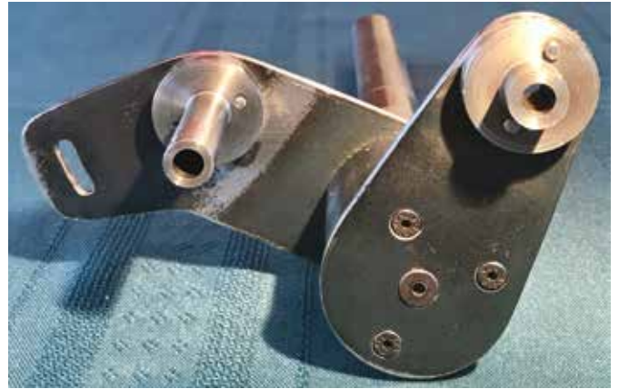
Figure 6. The two supporting plates attached to the main boss. The distal plate is fixed to the main boss by one central and three radially disposed 3 mm socket-head cap screws. The two bearings for the drive and lead-screw shafts are of cast iron, which has the excellent property of retaining oil in such bearings.
