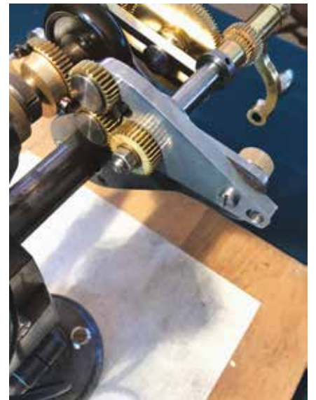
Figure 13. Close up of the tumbler (direction-reversing) wheels on their platform.
