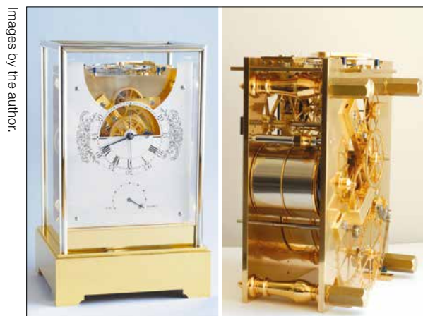
Figure 9. Harrison's H4/H5 mechanism reconstructed in an eight-day clock with Tensator mainsprings. The component parts from the centre wheel on through the train, copy the originals, although the arbors are extended to correspond with the separation of the plates. The Tensator springs provide an almost constant drive, similar to the fusee system that Harrison used in H4/H5 and include his maintaining power. The reserve of going indication has been added for convenience.
