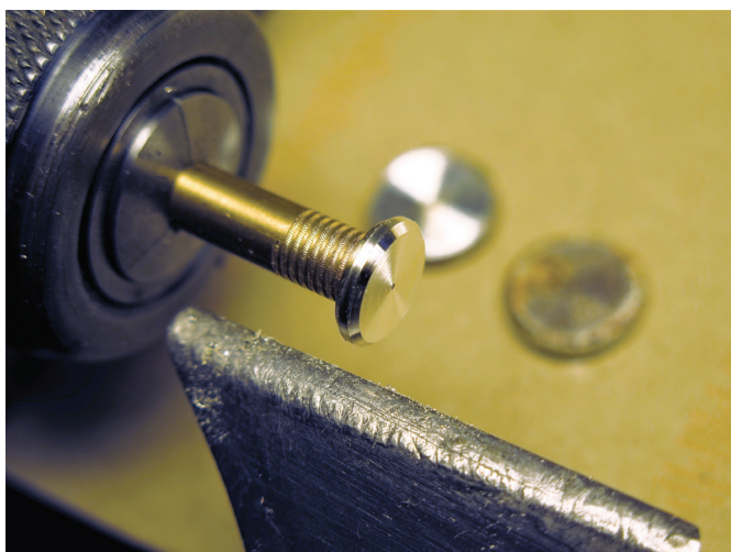
Figure 12. Turning the button to size, in the background one button hammered flat, the other part turned.
