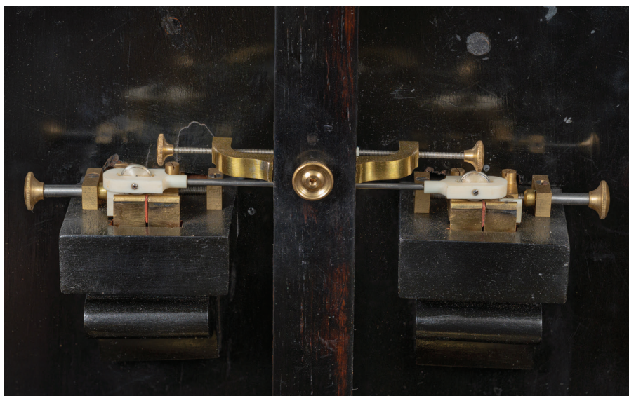
Figure 9. Clock Two; much of the contact assembly was missing. The replacements were made longer by about two millimetres to prevent the trolley running off, as sometimes experienced with Clock One.
