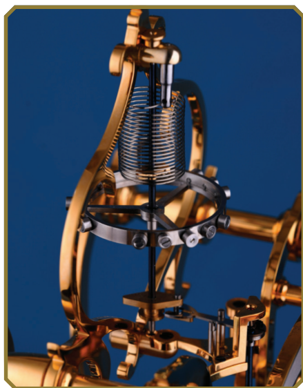
The clock train emulates antique Condliffs, beating seconds; this is an adaptation of the Sinclair Harding version that beats \frac{1}{4} seconds. Lever escapement with helical balance spring and jewelled balance bearings.
