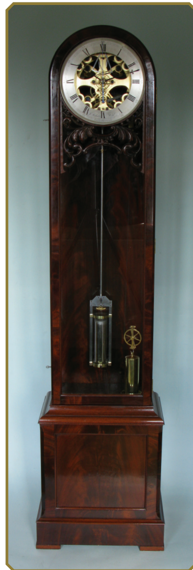
Gravity-escapement regulator, with mercury pendulum; the case purpose-made for the clock by an English clock-case maker in the Victorian style.
