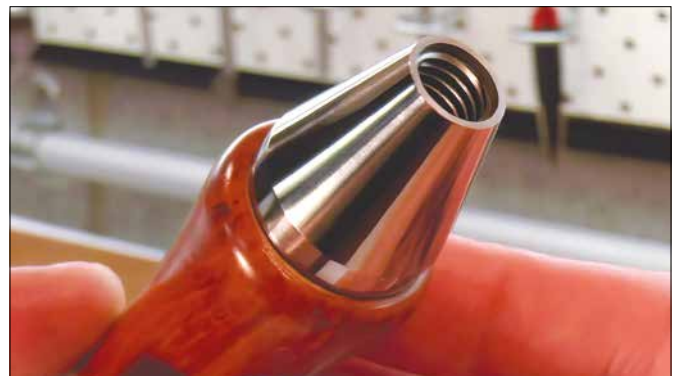
Figure 9. The part is tapped home into a suitable handle.
