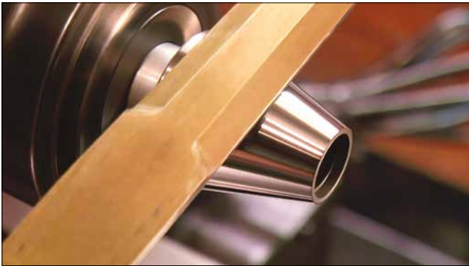
Figure 7. Polishing permits observation of the tempering colours.
