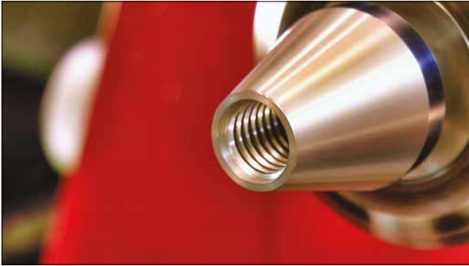
Figure 5. Note the undercut at the start of the thread.
