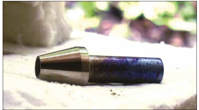
Figure 8. Running the oxide colours up from the shank section.
