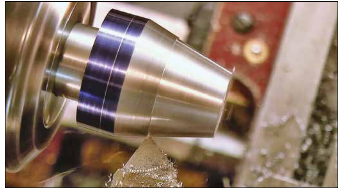
Figure 4. Set up for an included angle of 30 degrees.
