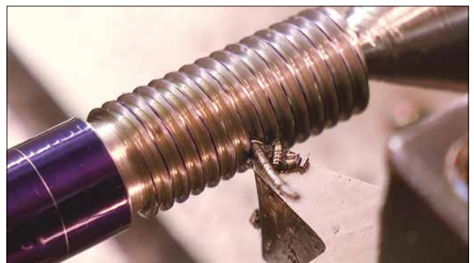
Figure 20. The top-slide (assuming a 60 degree thread) is set to 29.5 degrees.
