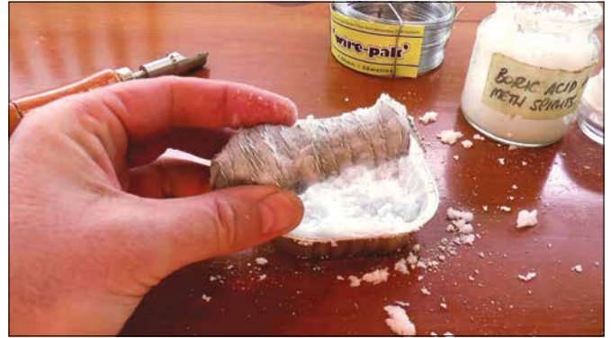
Figure 6. Wire and powdered boric acid paste is applied.
