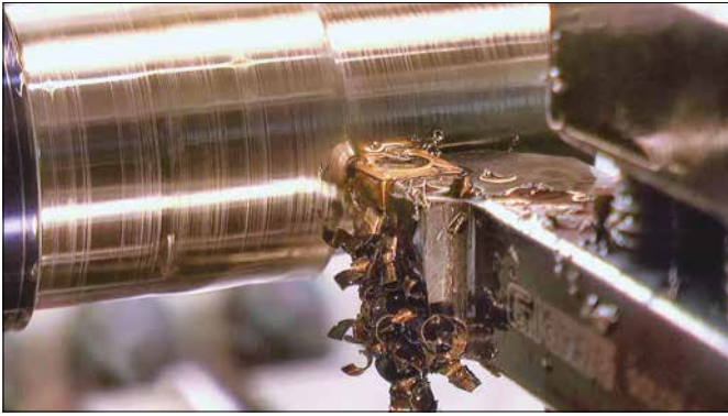
Figure 3. Switching to carbide inserts for the bulk stock removal.
