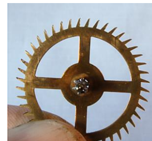
Figure 88 – tooth form of escape wheel
