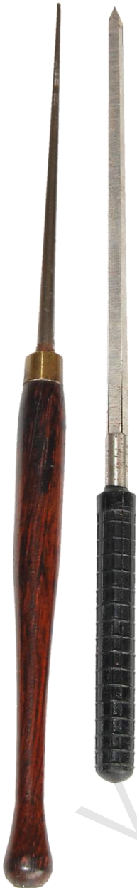
Figure 131 – smoothing broach (left), and cutting broach
