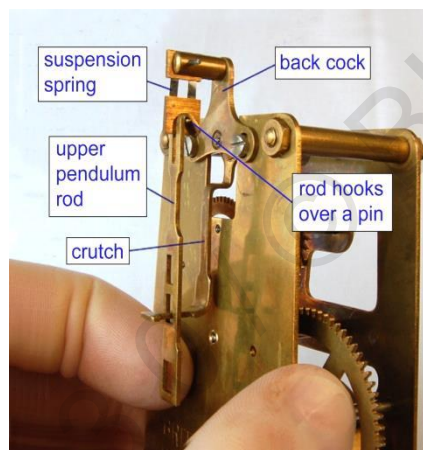
Figure 65 – mounting the pendulum
