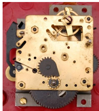
Figure 36 – movement of Japanese alarm clock
