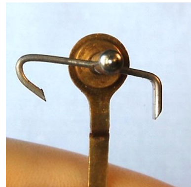
Figure 70 – close-up of pallets
