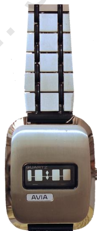
Figure 50 – very early LCD watch with 'random dispersal' display
