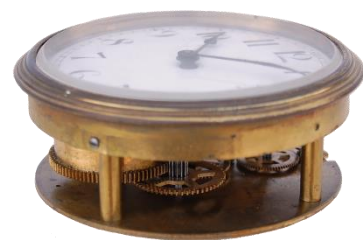
Figure 21 – another view, showing typical proportions of a drum movement
