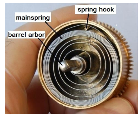
Figure 84 – barrel with end cap removed
