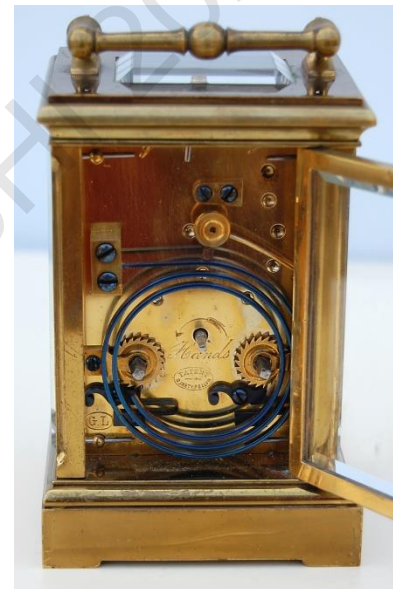
Figure 17 – carriage clock rear, showing attractive finish
