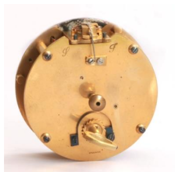
Figure 20 – drum movement showing platform escapement
