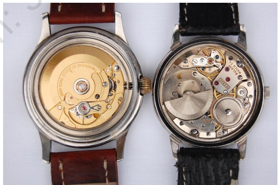
Figure 47 – 20th century ETA and Bulova movements
