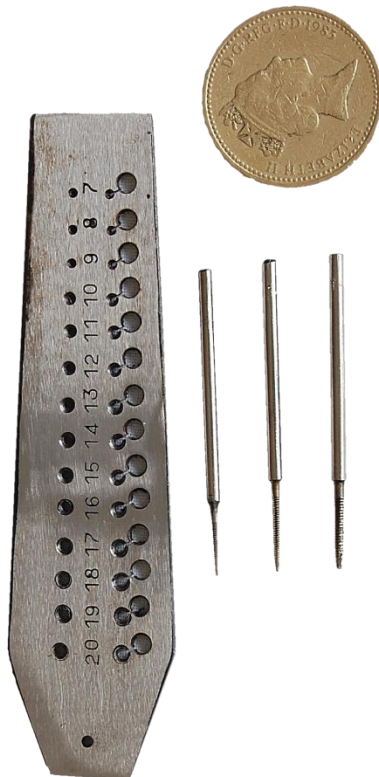
Figure 134 – screw plate and three watch-sized taps, with a pound coin for scale
