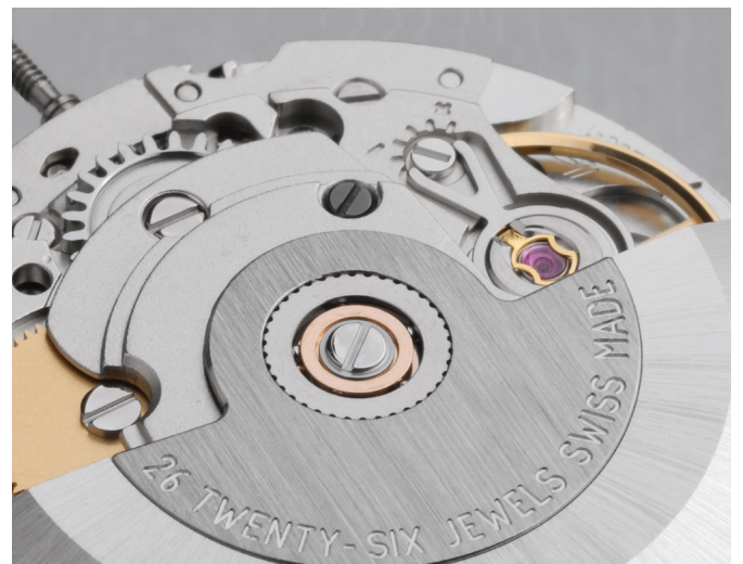
Figure 12. The Sellita SW200 movement, which powers anOrdain's watches.
