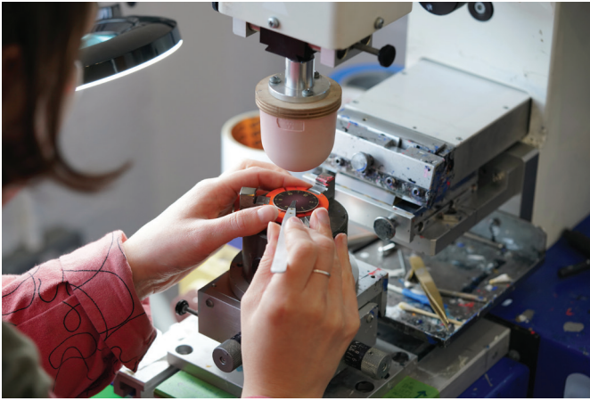
Figure 3. Enameller Morna Darling pad-printing a blank fumé enamelled watch dial.
