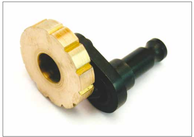
Figure 5. The Jacot drum and locator.
