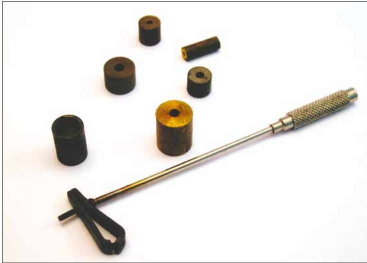
Figure 38. The small lighter fuel gas torch.
