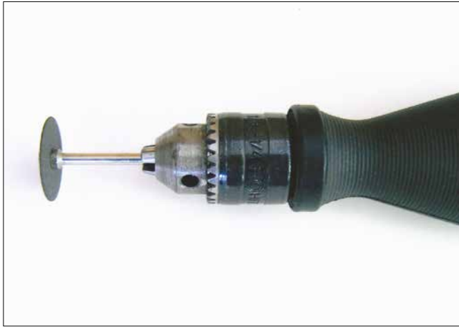
Figure 34. The blued pivot steel is cut with a Dremel or Multi-Craft with cut-off wheel.
