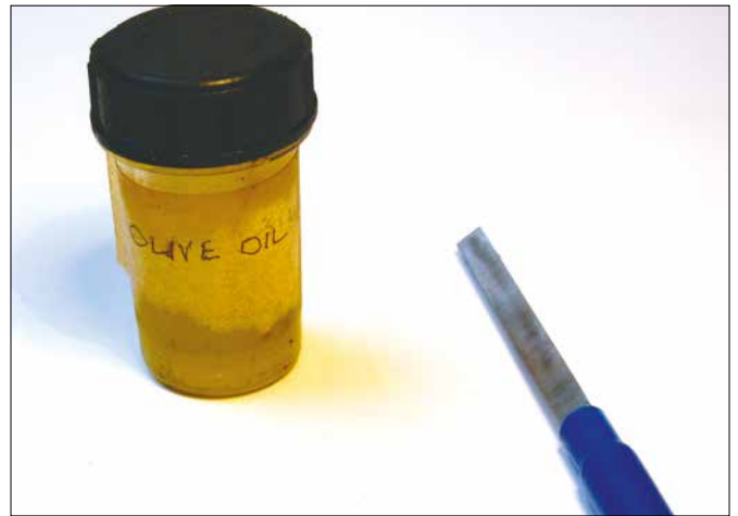
Figure 7. A lubricant is used on the burnisher.
