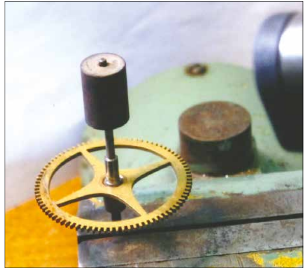
Figure 39. When softened, the arbor should be a nice blue.
