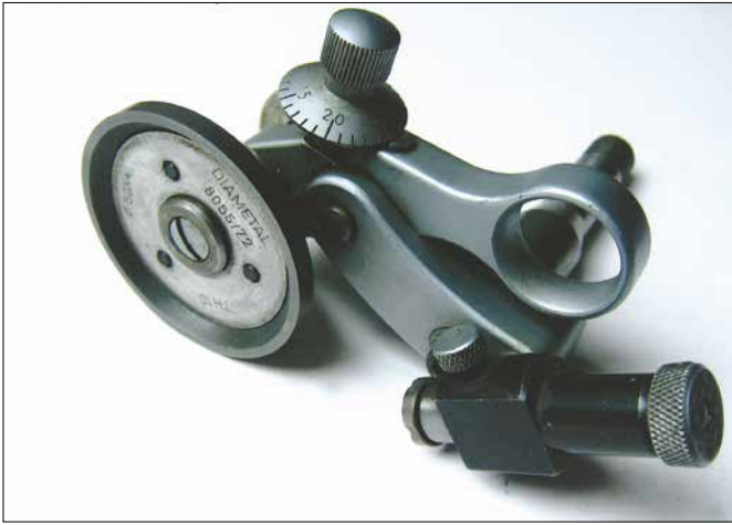
Figures 12 and 13. A burnishing tool by Bergeon.
