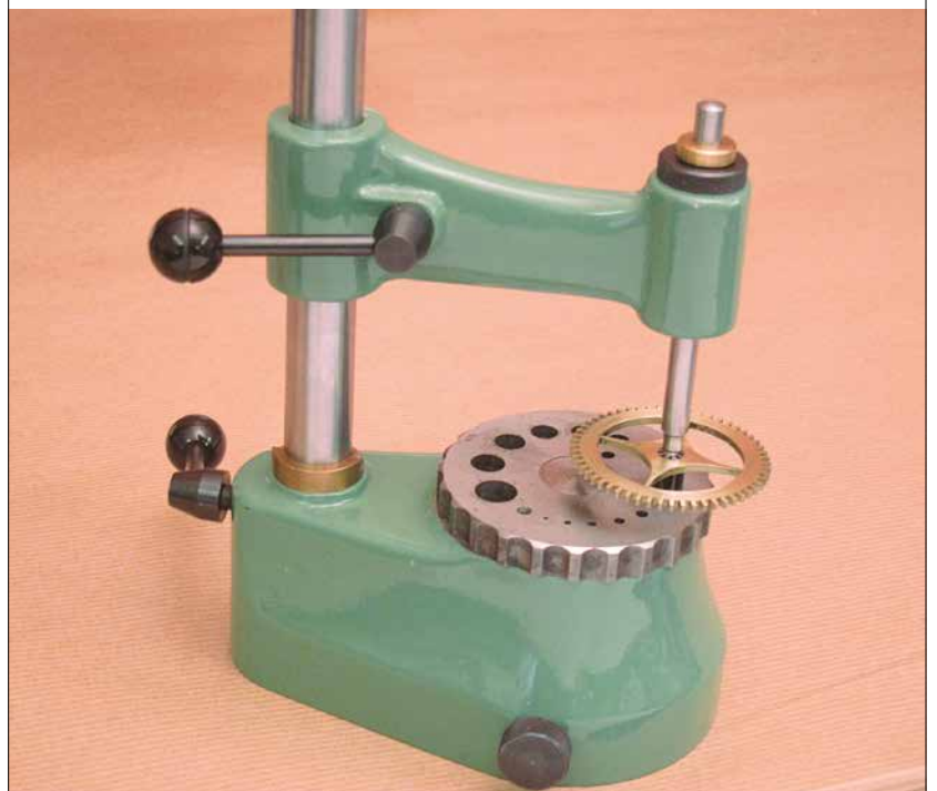
Figures 37A and 37B. Two methods of inserting the pivot materials: using the lathe tailstock with special runner or using a staking tool.
