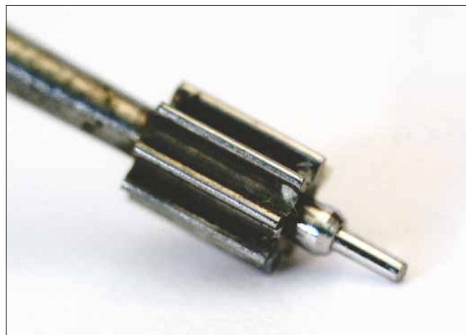
Figure 9. A completed pivot.
