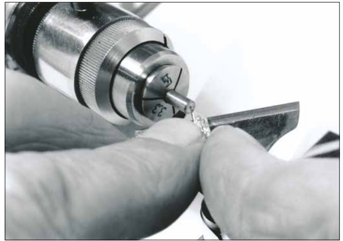
Figure 23. A centre being cut with the graver.
