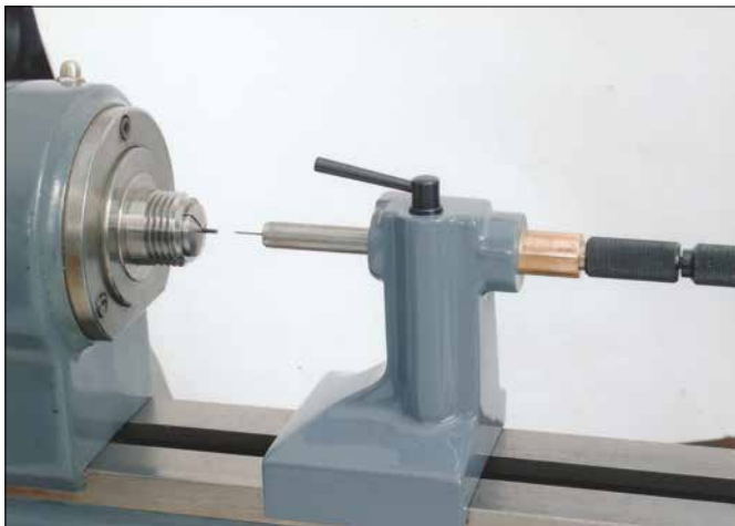
Figure 32. Using the tailstock the author made for the Schaublin 70 lathe.
