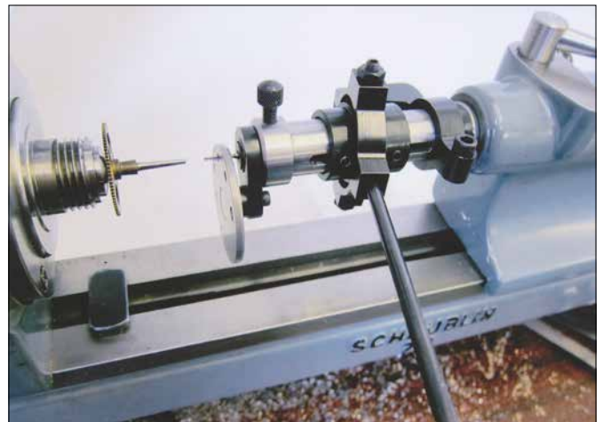
Figure 33. Using the new lever feed that retro-fits to the author's standard Pivot and Jacot Tool.
