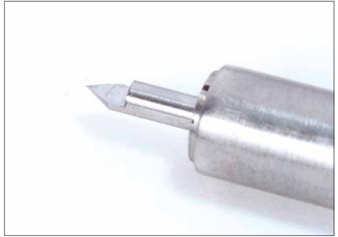
Figure 25. A homemade 'D' bit centre drill.
