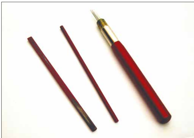
Figure 2. A sapphire burnisher and two Degussit stones.
