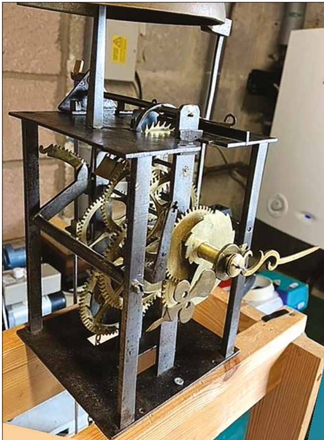
Figure 2. Ian Harris's restored 30-hour Comtoise movement.
