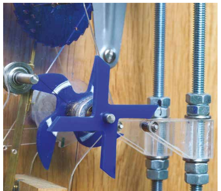
Figure 15. Close-up of the escapement from the left.
