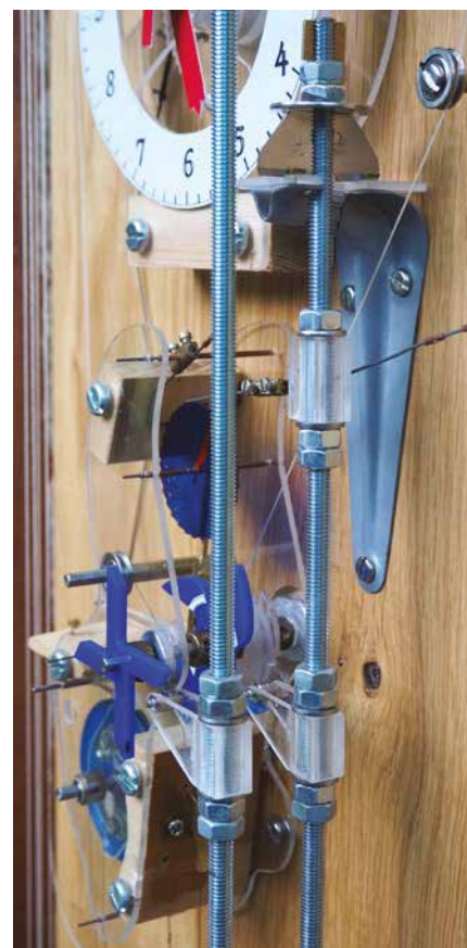
Figure 11. View from the right of the escapement, showing knife-edge pendulum suspension.
