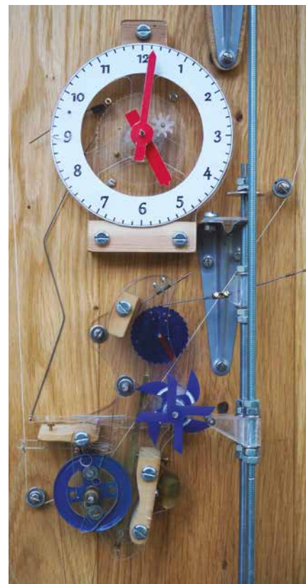
Figure 10. Enlarged view of clock layout. Note the Z-shaped wire pusher for advancing the minute hand and the Ferguson's paradox motion work behind the dial.
