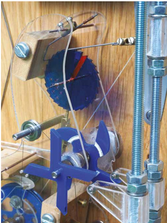
Figure 14. Close-up of the escapement. Pendulums free to swing with the cam arbor latched.
