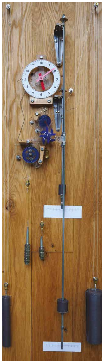
Figure 9. Overall view of clock layout, showing larger drive weights and smaller remontoire weights.
