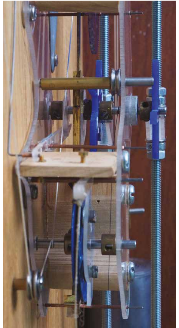
Figure 13. The escapement from the left. The white cord rewinds the remontoire and the black cotton thread, near the front of the mechanism and wrapped around the cam arbor, is the Huygens loop of the remontoire.
