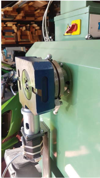
Figure 3. A small rotary table used to drive a lathe headstock to provide divisions. Image provided by Stephen Ward.
