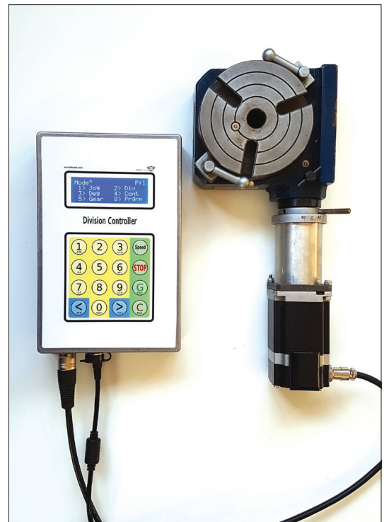
Figure 2. A stepper motor applied to a rotary table. Image provided by Stephen Ward.
