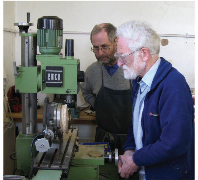
Figure 5. Cutting a 120-tooth escape wheel at Upton Hall. Pictured here are Tony Temple and the late Ken Johnson.
