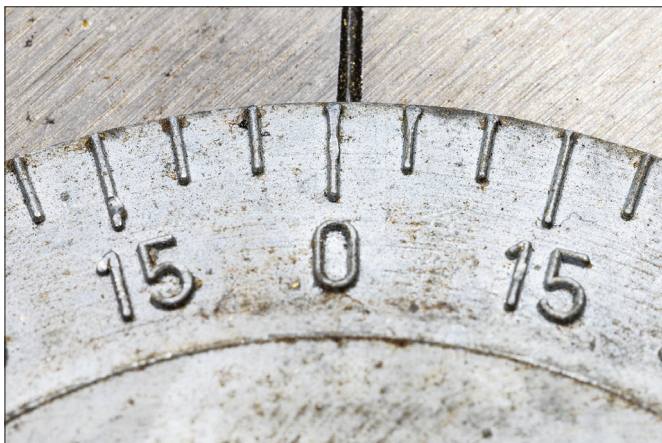
Figure 6. The graduations for the top slide are 5^\circ . It is difficult (impossible?) to accurately adjust the slide to 0.295^\circ .
