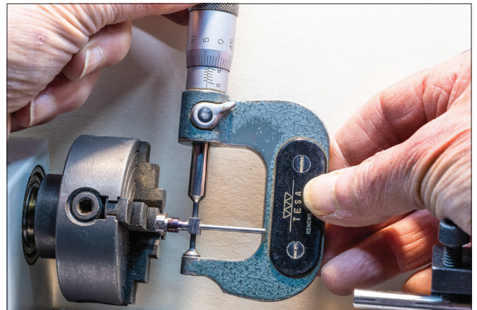
Figure 24. Measure the distance across flats in both directions and check whether the flats meet at the corners.
