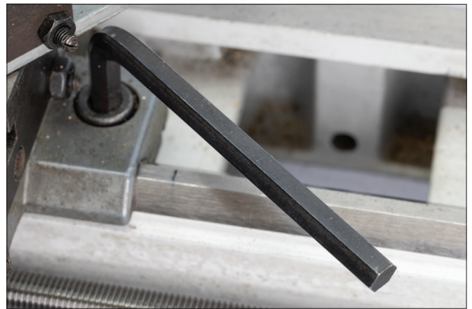
Figure 16. Always lock the carriage when it is not being moved. This gives greater rigidity.
