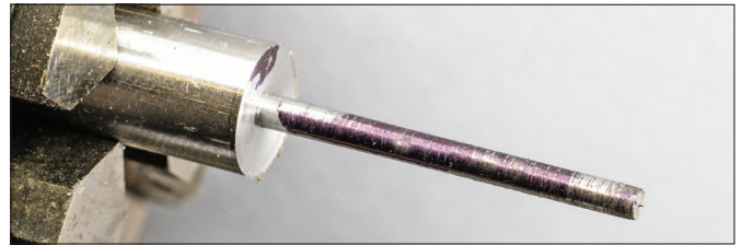
Figure 19. The felt tip is rubbed away at points along the length of the taper.
