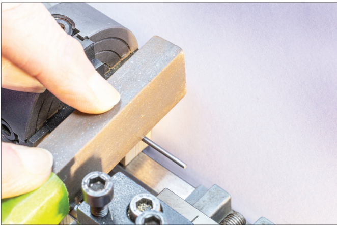
Figure 25. Ensure the oilstone is pressed firmly against the square and the silver steel held in the tool post.
