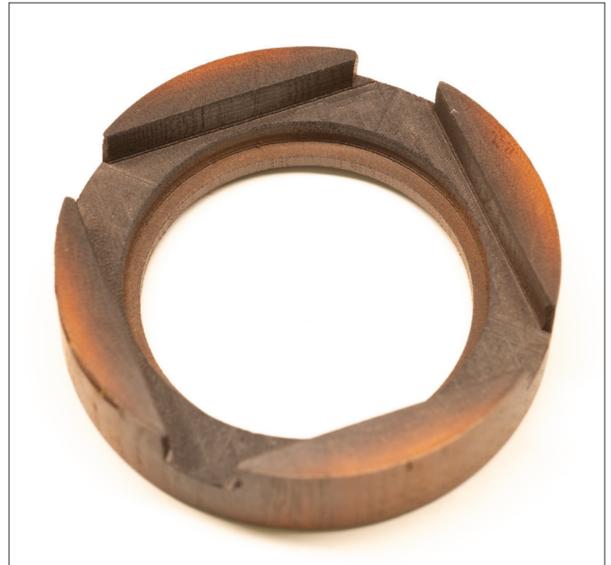
Figure 1. A phenolic frame (shown here upended) to sit over the hotplate, capped by a watch glass to create a heating chamber.
