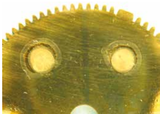
Figure 4. Visual evidence of corrosion on the brass plate was apparent.
