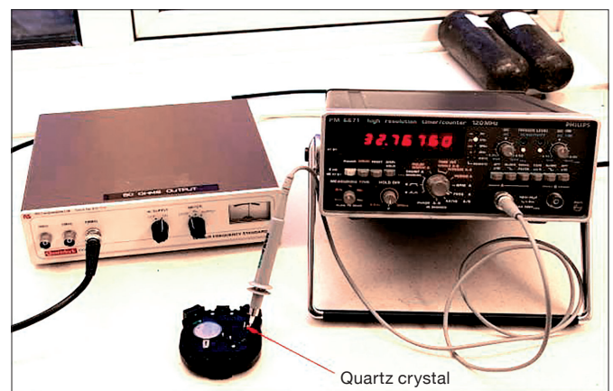
Figure 4. An off air standard and frequency counter with quartz watch. Losing one second per day.
