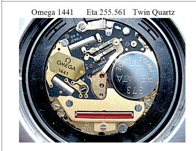
Figures 2A and 2B. The Omega Cal. 1441 showing twin quartz crystals and digital pulse inhibition contacts.
