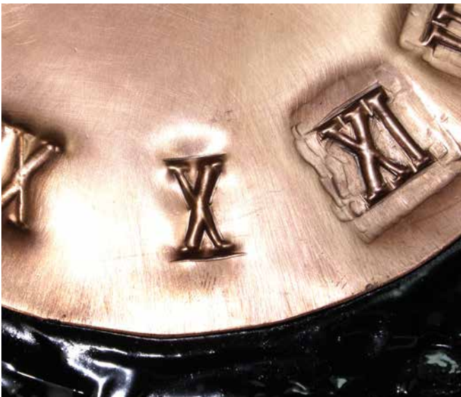
Figure 13. How the numbers are sharpened by chasing.
