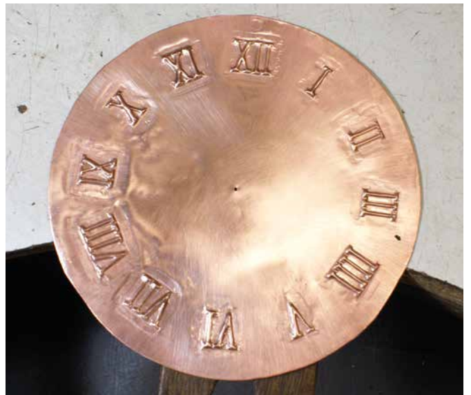
Figure 14. The disc with chasing complete.
