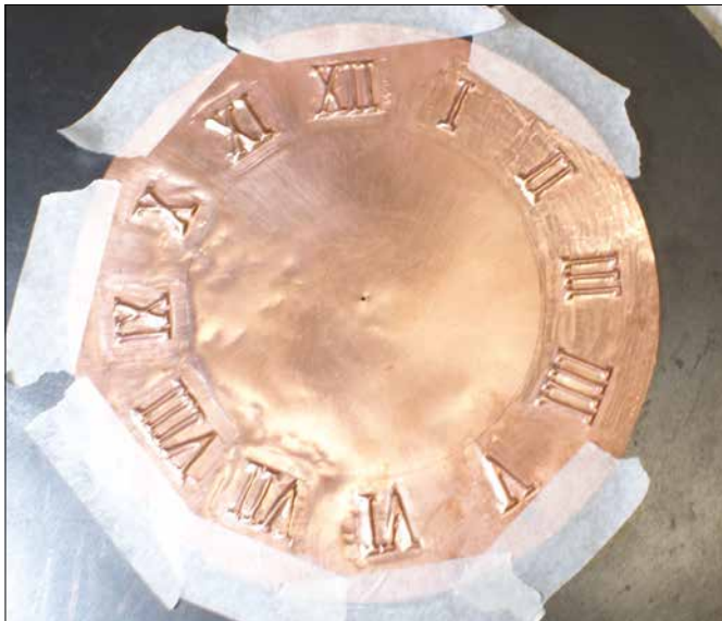
Figure 15. Planishing the background on a steel plate.
