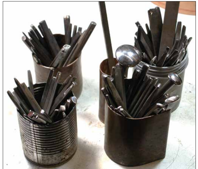
Figure 6. A range of punches.
