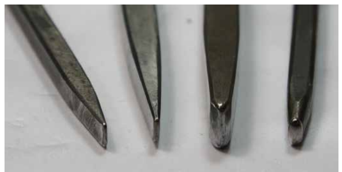
Figure 5. The basic punches.
