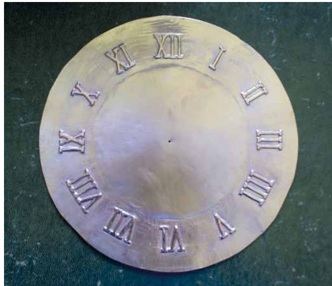
Figure 16. The numbers planished and burnished.
