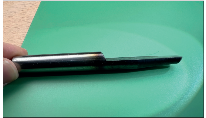
Figure 3. A wheel riveting tool - milled, hardened and polished.
